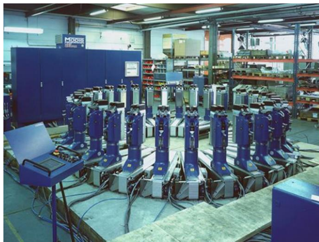
Figura 7: Utillaje flexible UHF-Chord Trimmer.
