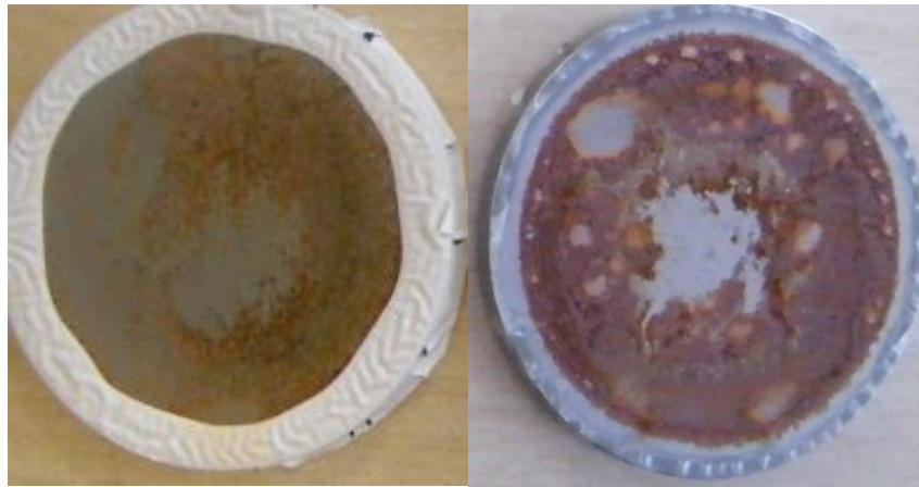
Figure 3.12 Samples #350.5 (left) and #350.25 (right) at the SST test after 4h.
