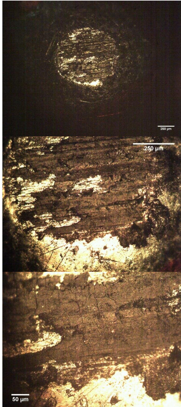
Figure 4.48. Micrographs of the wear track on the Al ball sliding against coating ref #DLCCH after the electro-tribology test.
