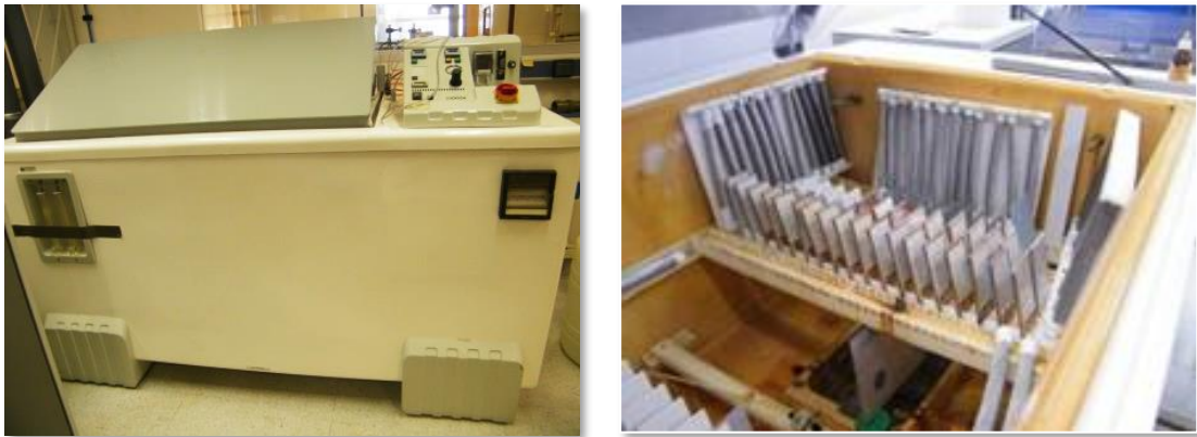
Figure 2.27. Salt Spray Test Chamber and sample lay-out.
