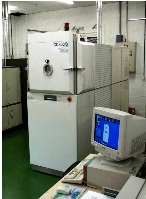
Figure 2.13. CEMECON CC800/8 plus PVD equipment.
