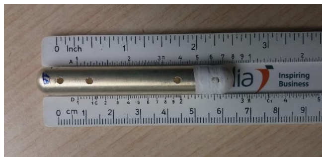
Figure 2.25. Image of one of the Ag coated Cu pins used as counterparts in the electro-tribological studies against AgAl coatings.
