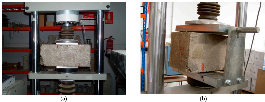
Figure 4. (a) UCS test; (b) indirect tensile strength (ITS) test.
