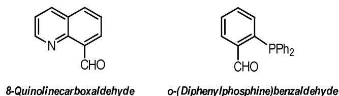
Figure 33. Structures of chelating aldehydes C_9H_6NCHO and PPh_2(o-C_6H_4CHO) .
