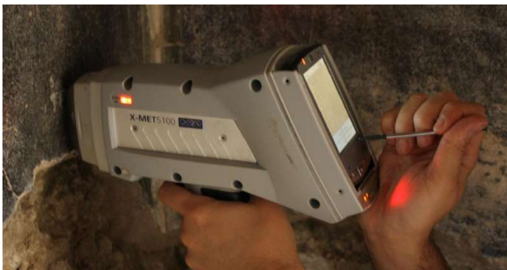
Fig 3.6. The X-MET 5100 handheld EDXRF spectrometer measuring a Pompeian wall painting.
