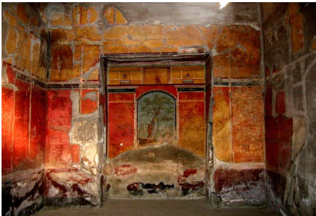
Fig. 11.1. Wall painting from Herculaneum showing original yellow, incomplete transformation (orange areas) and complete transformed yellow into red areas 1 .
