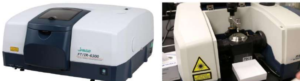
Fig 3.9. The Jasco 6300 infrared spectrometer (left) and ATR module integrated in it (right).
