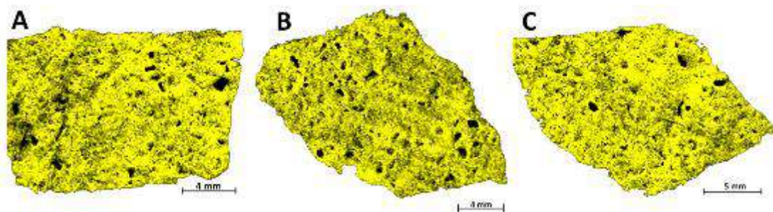
Fig. 11.9. Iron distribution XRF maps (in yellow) in A, B and C fragments.
