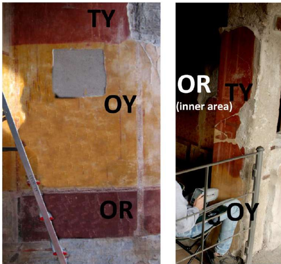
Fig. 10.3. Wall paintings on the House of Marcus Lucretius (left) and House of Gilded Cupids (right) showing the in situ analyzed three areas. (OR: Original red; OY: Original yellow; TY: Transformed yellow).
