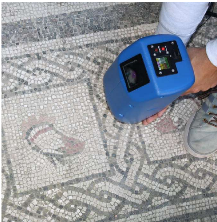
Fig 3.7. EasyLIBS (model Easy 2C) handheld spectrometer from IVEA, measuring a mosaic from Pompeii.
