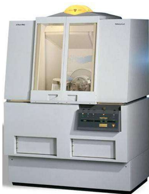
Fig. 3.10. PANalytical Xpert PRO powder diffractometer.
