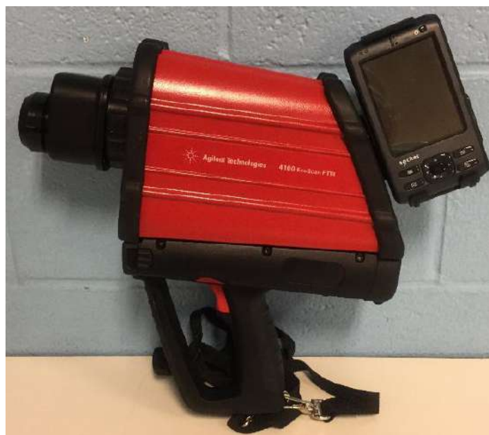
Fig 3.4. 4100 Exoscan handheld DRIFT spectrometer.
