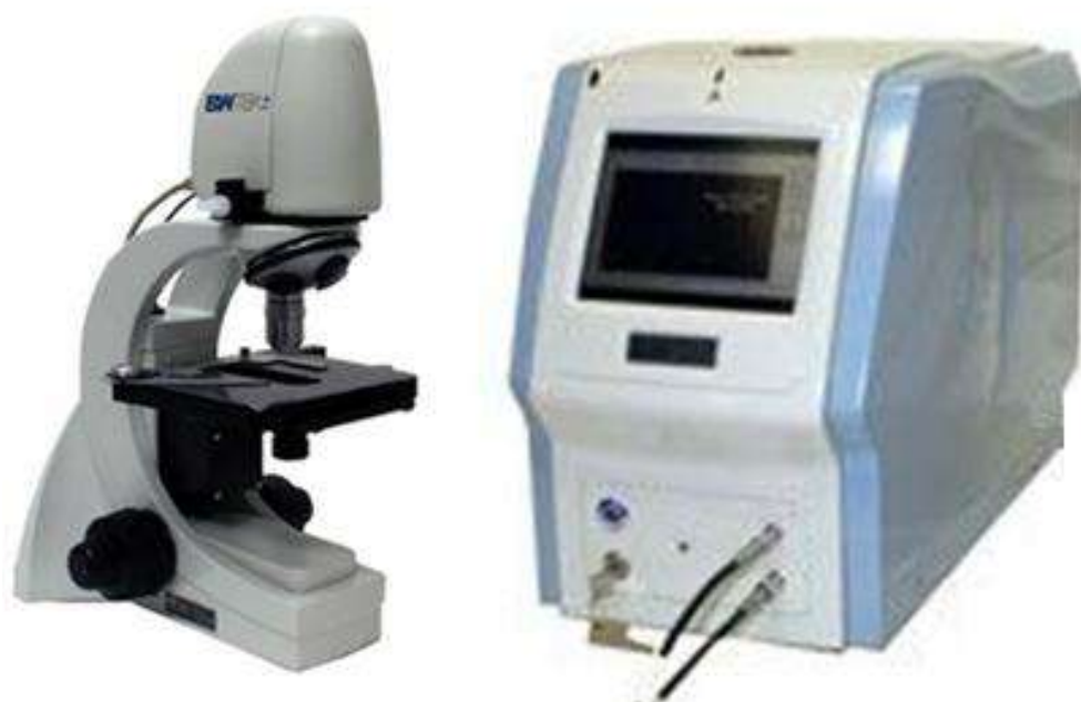
Fig 3.3. The innoRam portable Raman spectrometer with the used video-microscope.
