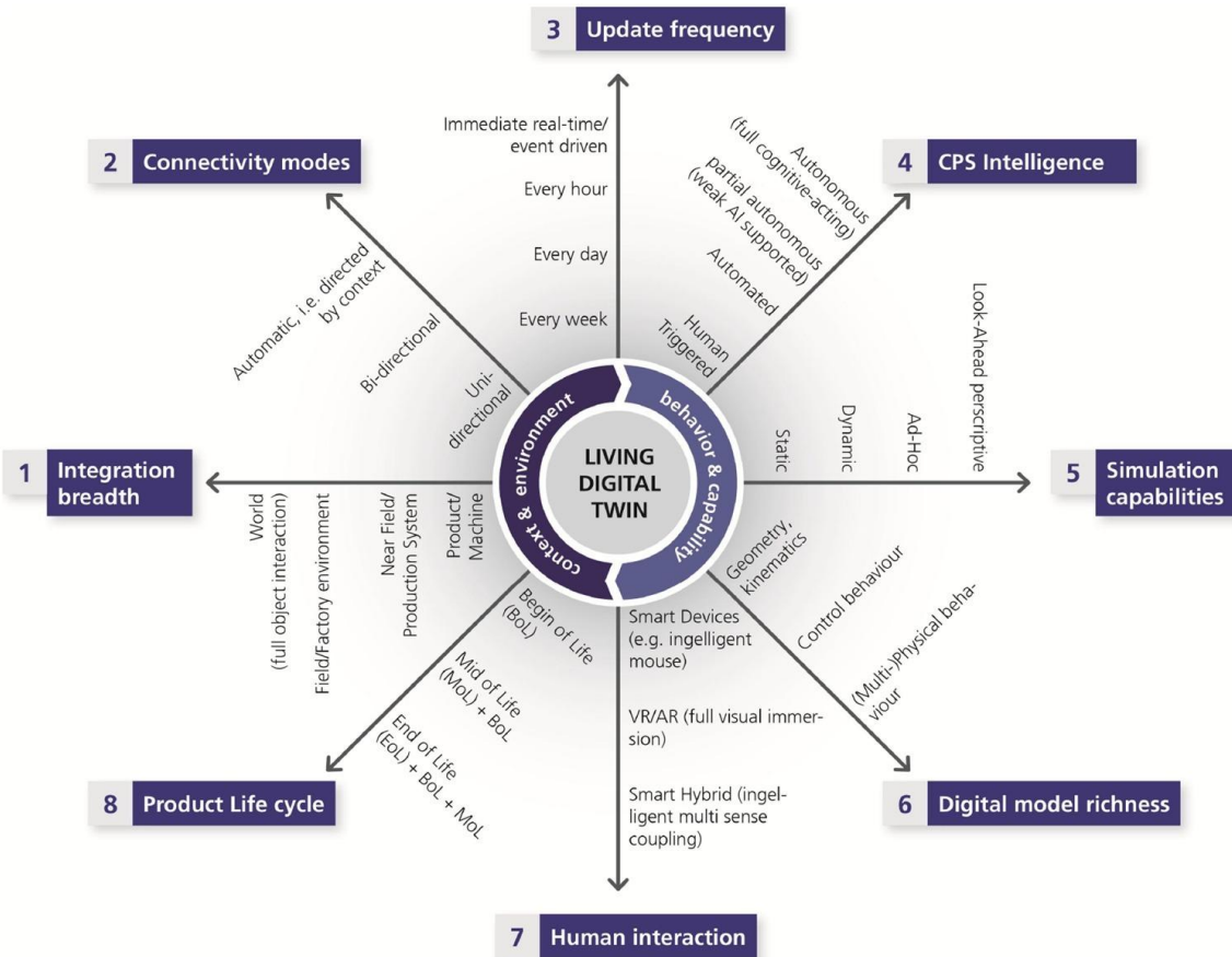
Figure II.36 Digital twin 8-dimension model (Stark R., 2019)
