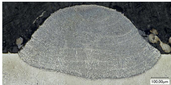
Figure IV.21 Microstructure from LMD Inconel®718 clad generation (UPV/EHU)
