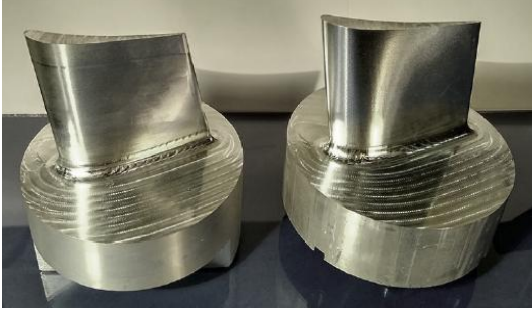
Figure V.9 Final obtained components using the default (left) and the algorithm (right)
