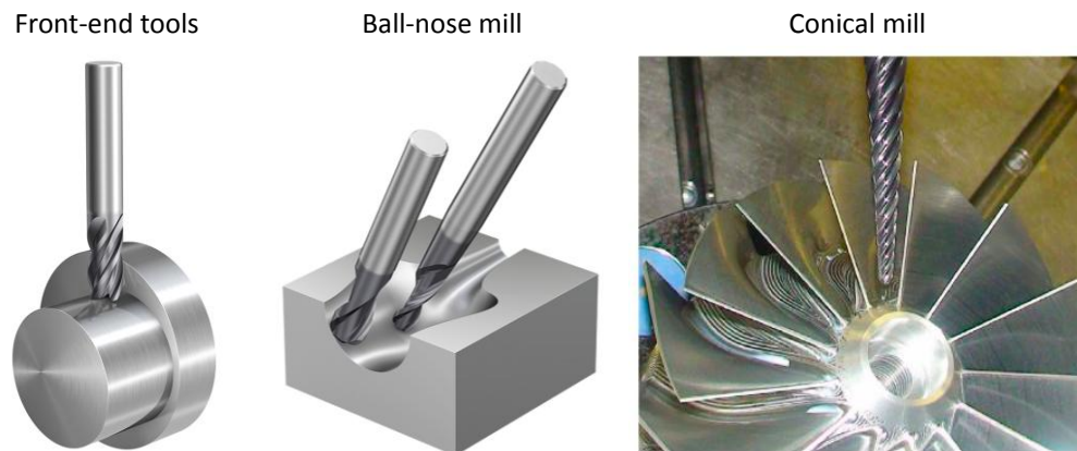
Figure II.23 Sandvik and Emuge-Franken milling cutting tool forms for IBRs manufacturing
