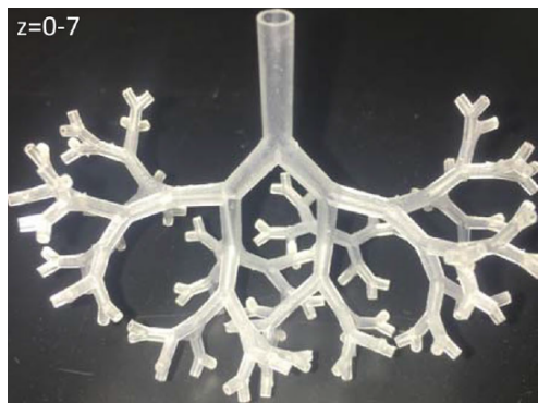
Figure 3.2: Eight-generation neonate airway model created with additive manufacturing techniques by Copploe et al.[126].
