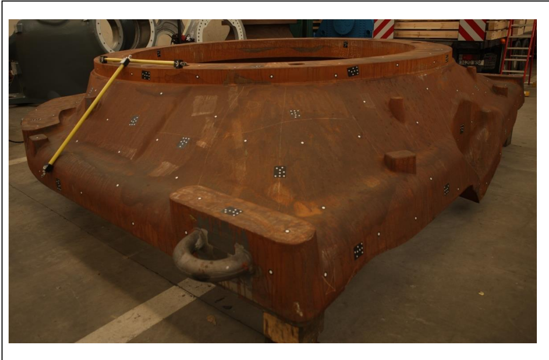
Figure 45. Preparation of the measuring object with targets (coded and uncoded) and calibrated bars
