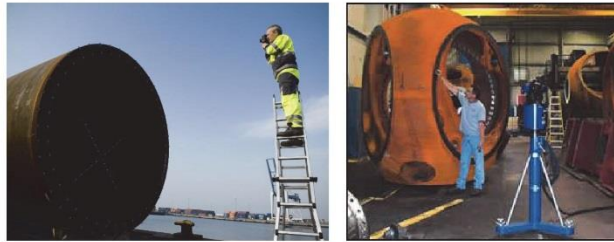
FIGURE 1: Standard procedures for machined part geometrical verification (from Zebicon & Modern Machine Shop).
