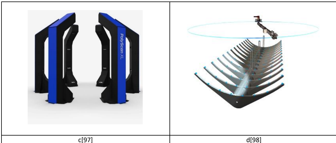
Figure 13. Fixed multi-view 3d scanning approach (a), measuring cell for tube inspection (b) industrial fixed 3D scanner (c) and customized multi-camera photogrammetric station
