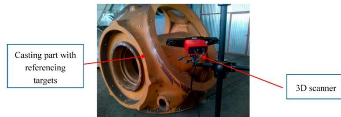
Figure 3. Scanning of casting part by means of structure light scanner and reference targets.
