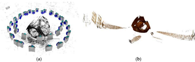
Figure 10. Dense matching schema for shop-floor case study: (a) structure from motion; and (b) dense 3D colored point cloud without filtering.
