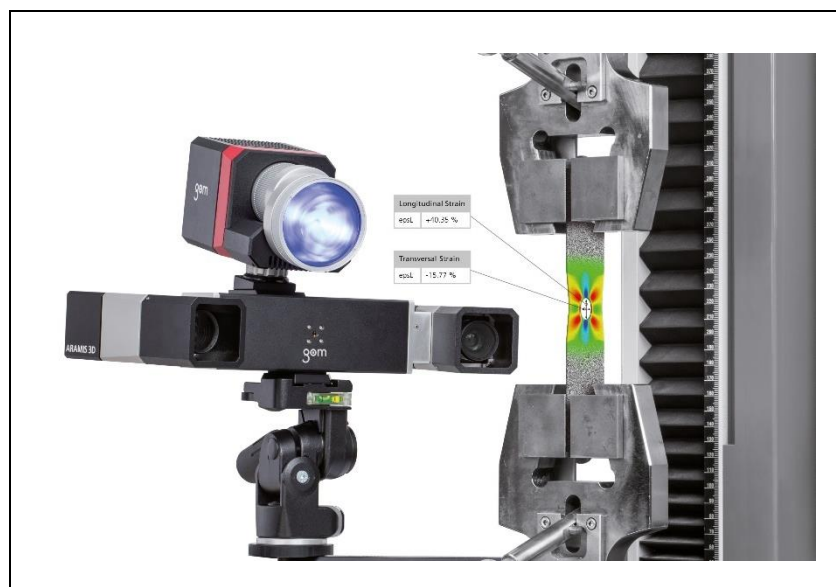
Figure 8. Digital image correlation for strain measurement[65]
