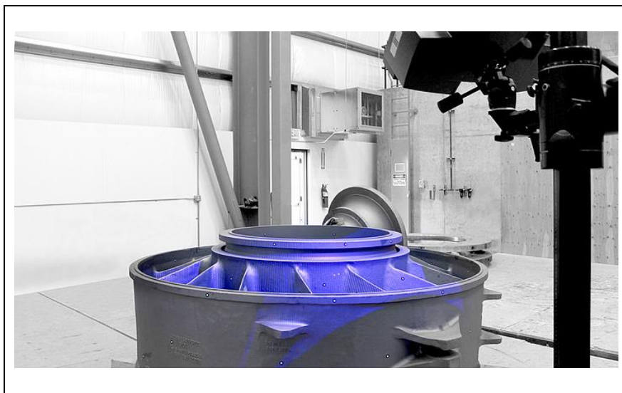
Figure 5. 3D optical scanning of casting parts with referencing targets[12]
