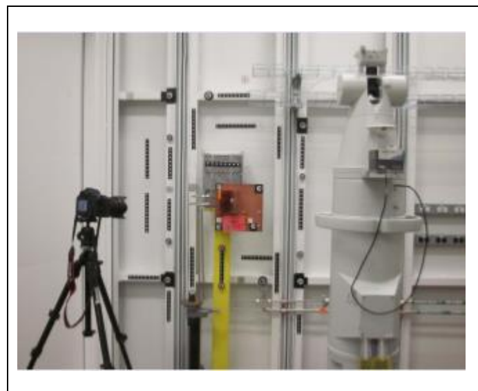
Figure 23. Portable coordinate measuring machines for structural health checking of CERN facilities.
