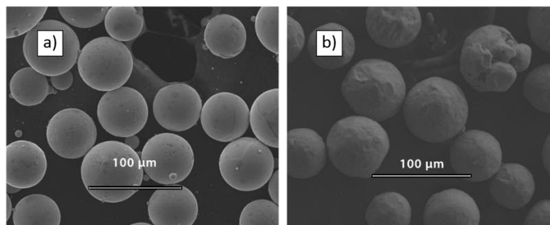
**Figure 8.** SEM images of (a) new Ti6Al4V powder, (b) strongly reused Ti6Al4V powder after the 69th cycle [125].
