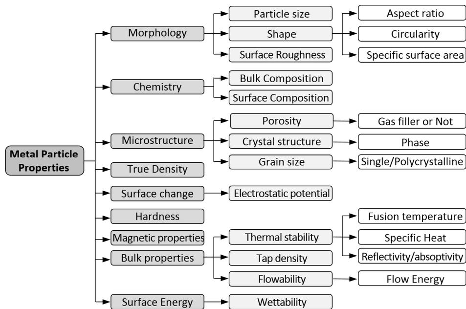
**Figure 9.** Classification of key metal particle properties that may influence AM part formation quality. Adapted from [127].
