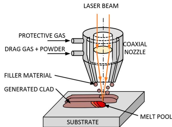
**Figure 2.** Basis of the LMD process.
