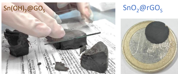
Figure 4.2. a) SnO 2 -rGO 3D foam and b) SnO 2 -rGO self-standing and binder free electrode.
