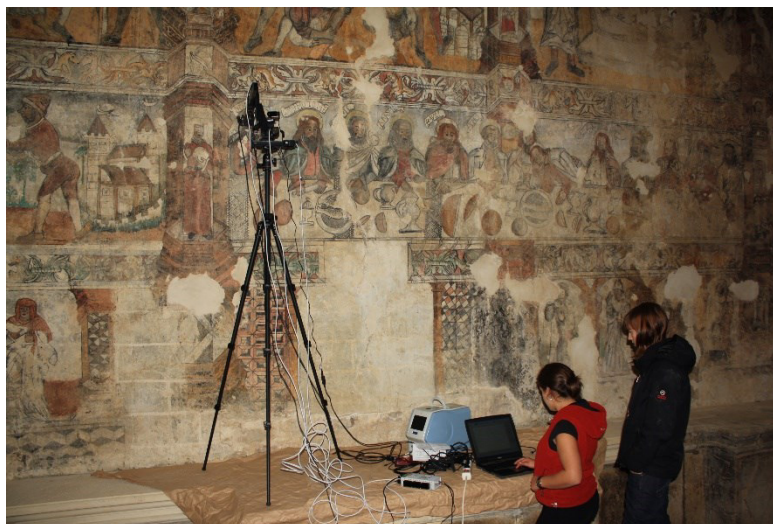
Figure 1.4: In situ Raman analysis of the medieval wall paintings located in the Saint Andrew Church (Biañez, Basque Country).
