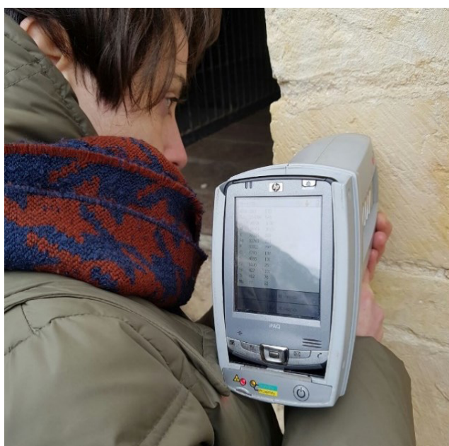
Figure 4.4: Use of portable ED-XRF instrumentation on the structural walls of Saint Stephen's church (Ribera de Valderejo, Álava).
