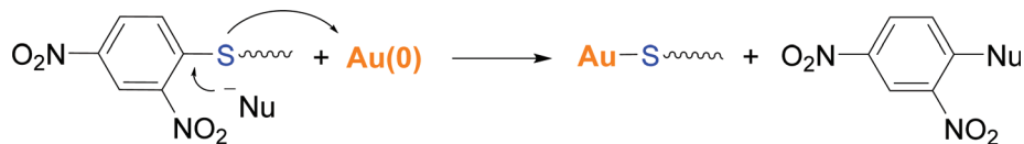
Scheme 3 The proposed reaction mechanism of gold modification with the 2,4-dinitrobenzene-protected thiol group.
