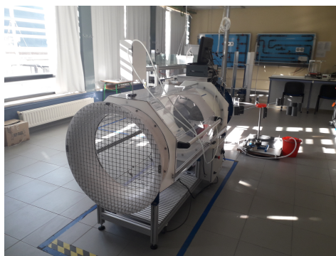
Figure 1. Windpump behind wind tunnel in fluid-mechanics laboratory at Engineering School of Gipuzkoa (Eibar).
