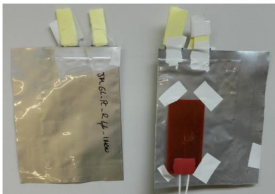
Figure 2.37. Polyamide Kapton Resistance placed between two Na-ion cells.
