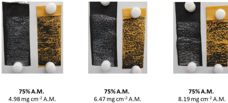
Figure 5.18. Aspect of the 75%AM electrodes with different AM loadings after the 180° peel test experiments.
