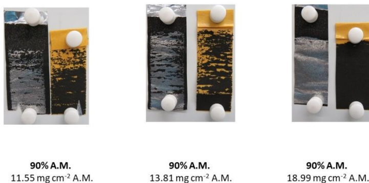
Figure 5.22. Aspect of the 90%AM electrodes with different AM loadings after the 180° peel test experiments.
