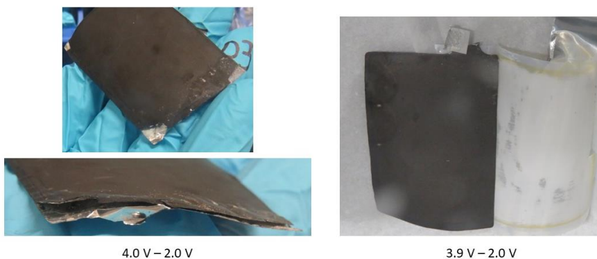
Figure 7.28. Visual aspect of the anode electrodes of S1.3_2.0-4.0 (upper cut-off voltage of 4.0 V) and S1.3_2.0-3.9 (upper cut-off voltage of 3.9 V) cells after cycling.
