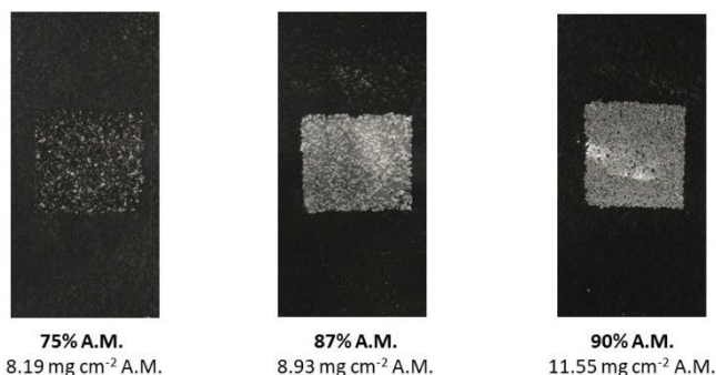
Figure 5.16. Electrode appearance after the adhesion strength tests.
