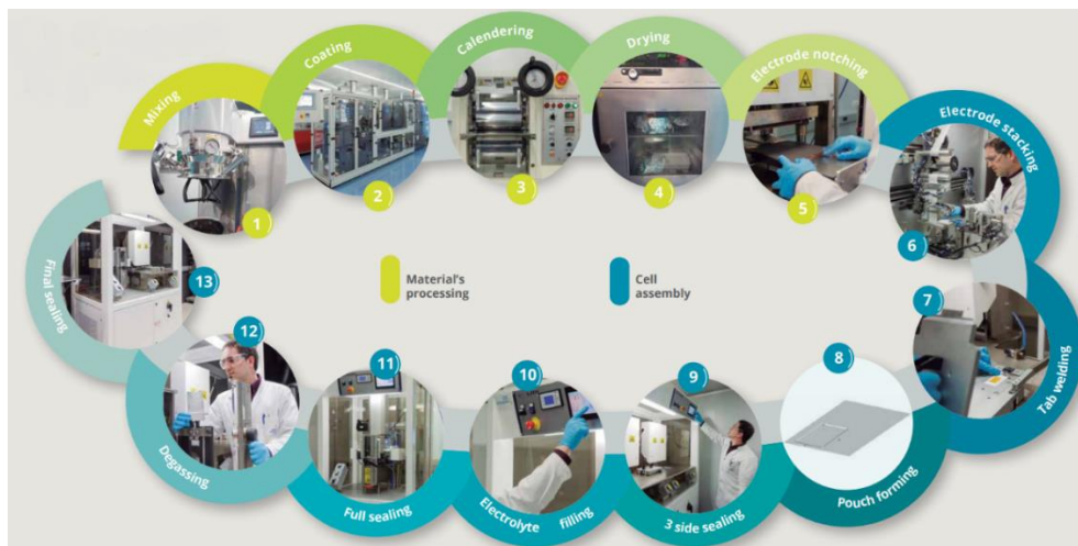
Figure 1.14. Illustration of Li/Na-ion cell manufacturing steps.
