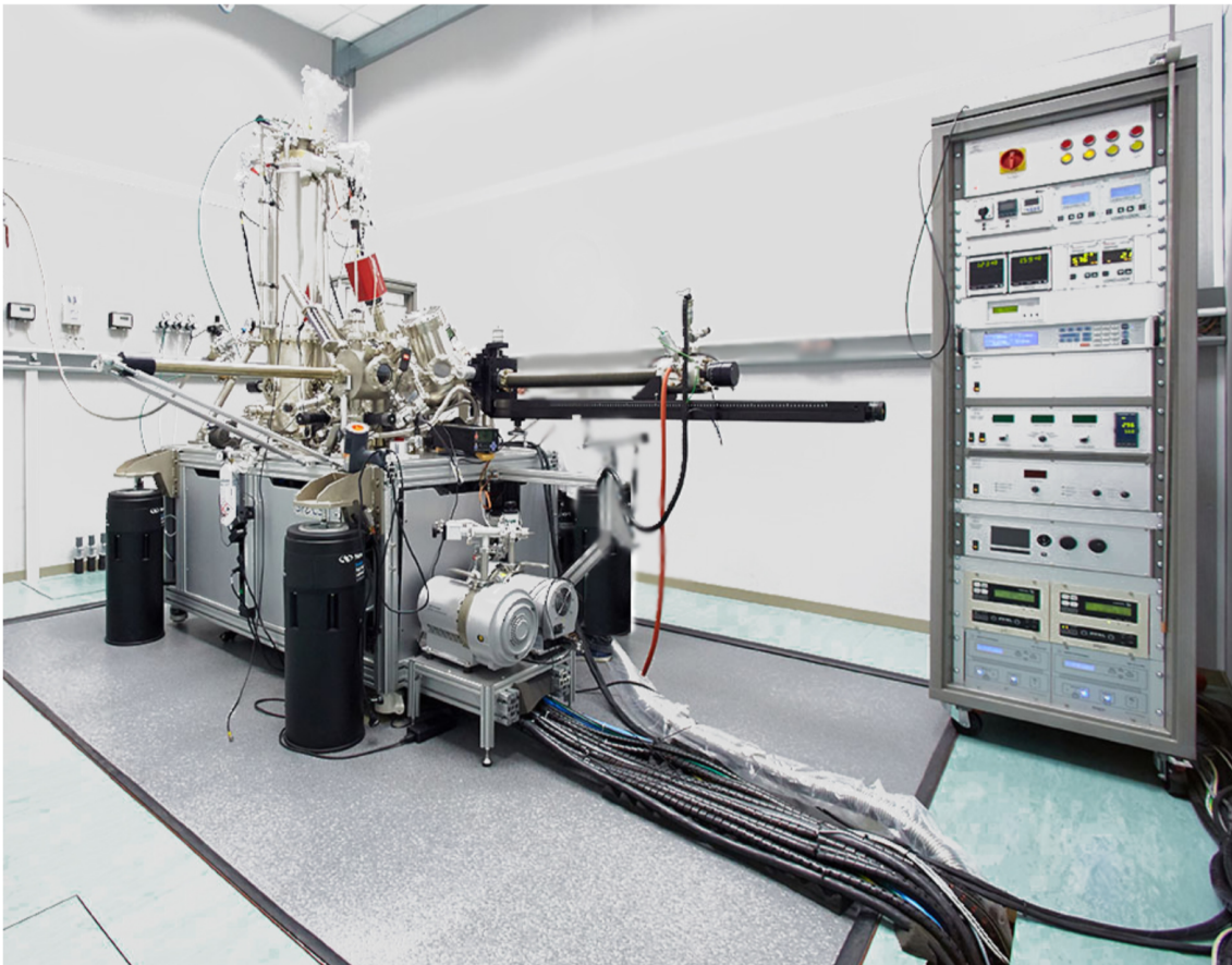
Figure 2.5: SPECS UHV-LT STM system. Picture of the STM system used in this work.
