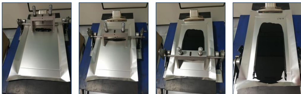
Figure 2.3. Casting of the LFP based laminate in the Doctor Blade.
