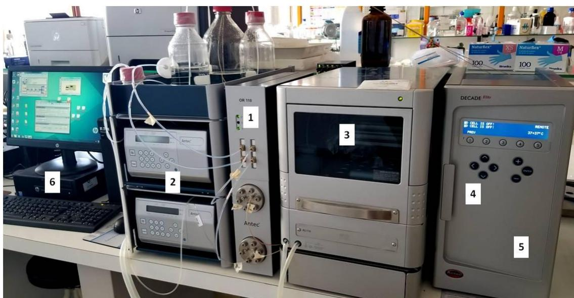
**Figure 3.25:** UHPLC equipment coupled to two electrochemical detectors. 1) Degasser; 2) Pump; 3) Autosampler; 4) Chromatographic columns; 5) Electrochemical detector; 6) Control station.
