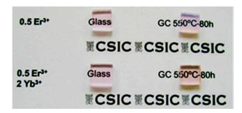
**Figure 1.** Transparent samples of  $0.5\text{Er}^{3+}$ -doped and  $0.5\text{Er}^{3+}$ -2Yb<sup>3+</sup>-codoped 70Si7Gd glass and glass-ceramics (GCs) heat-treated at 550 °C-80 h.
