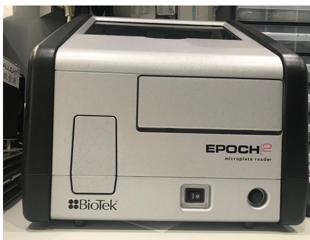
Figure 3.6. Spectrophotometer EPOCH 2 plate reader from BioTek.
