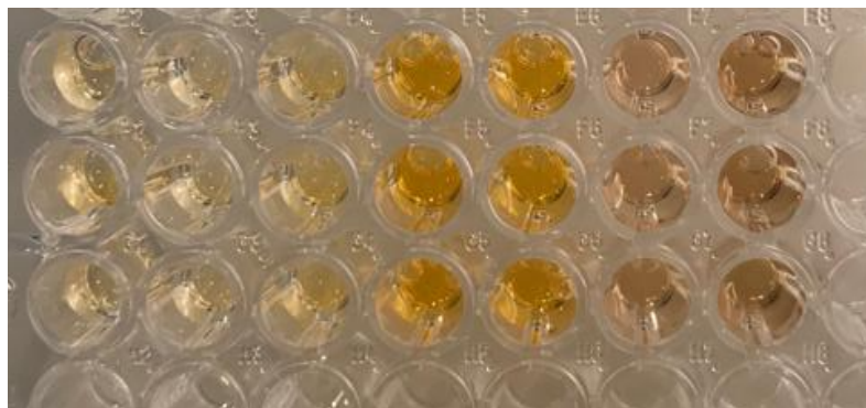
Figure 3.7. Example of a kinetic assay of DMP. The less substrate concentration the lighter orange we see. The experiment was carried out from 0.05 mM to 4 mM DMP.
