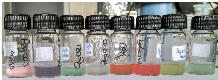
Figure 5.23. Nanoparticles suspension in MeOD after stirring 24 hours. From left to right; G6, G9, G12, G7, G5, G8, G4 and G10.
