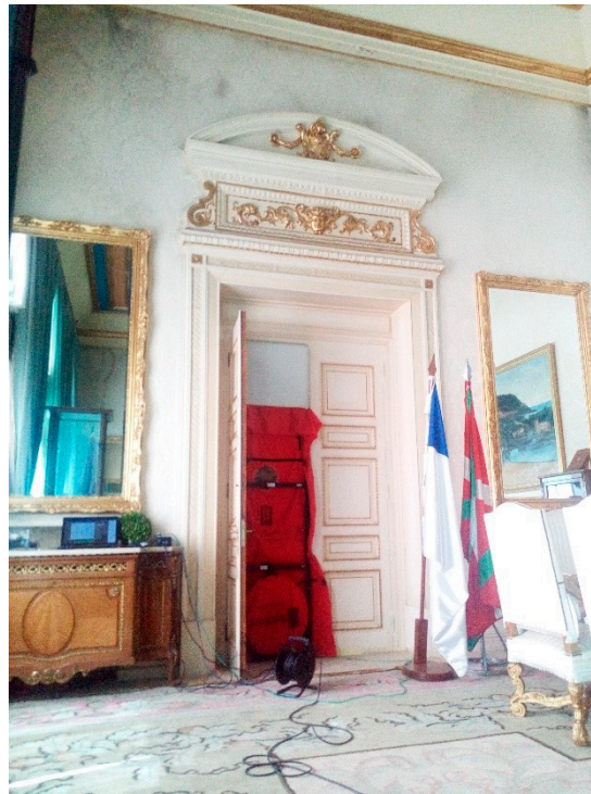
Figure 4. Use of the Minneapolis BlowerDoor equipment in the 31.F sample of the City Council building of Donostia-San Sebastián.
