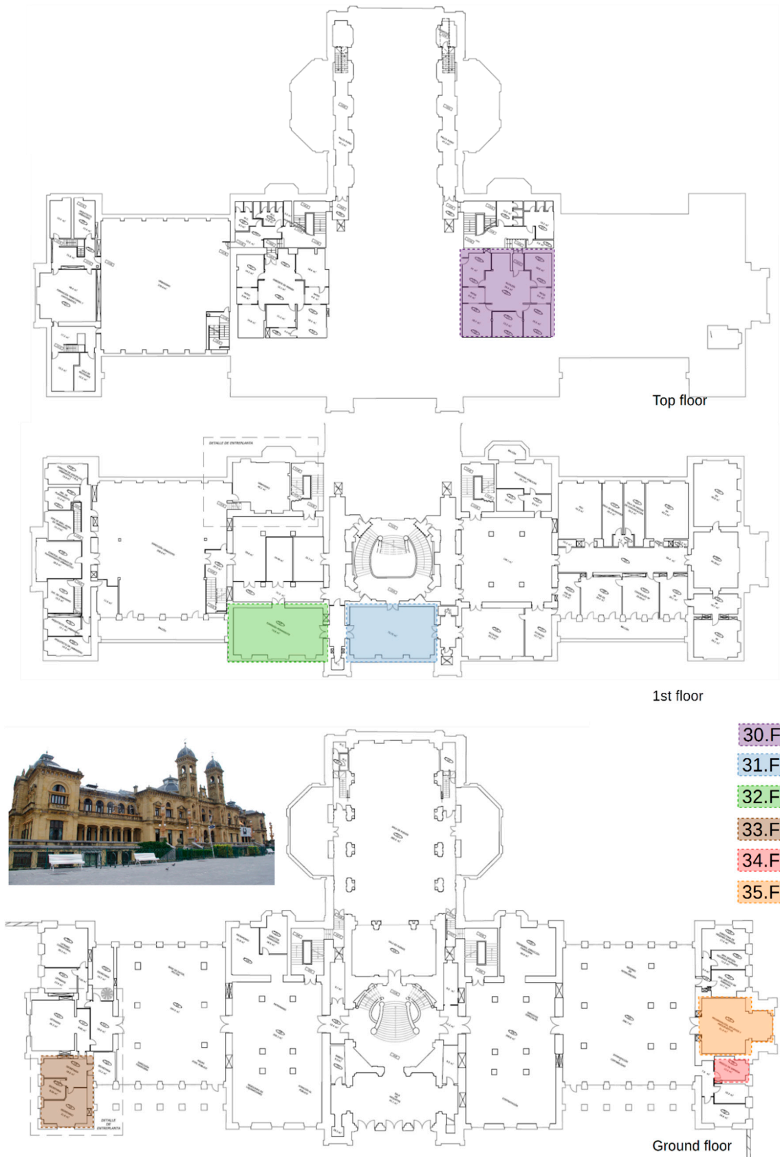
Figure A6. Floor plans of the blower door tests performed in the City-Council of Donostia-San Sebastián case study.
