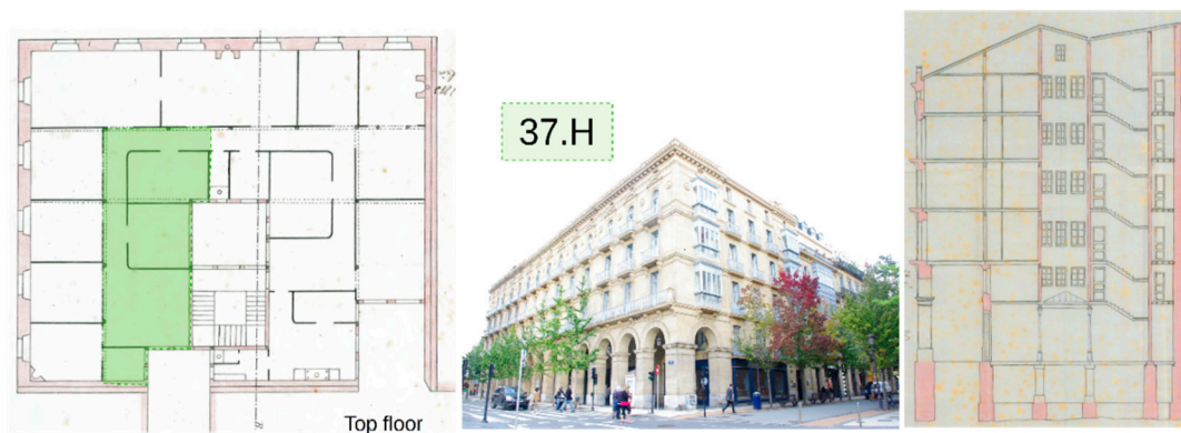
Figure A8. Floor plans of the blower door tests performed in the Loiola 14 case study.
