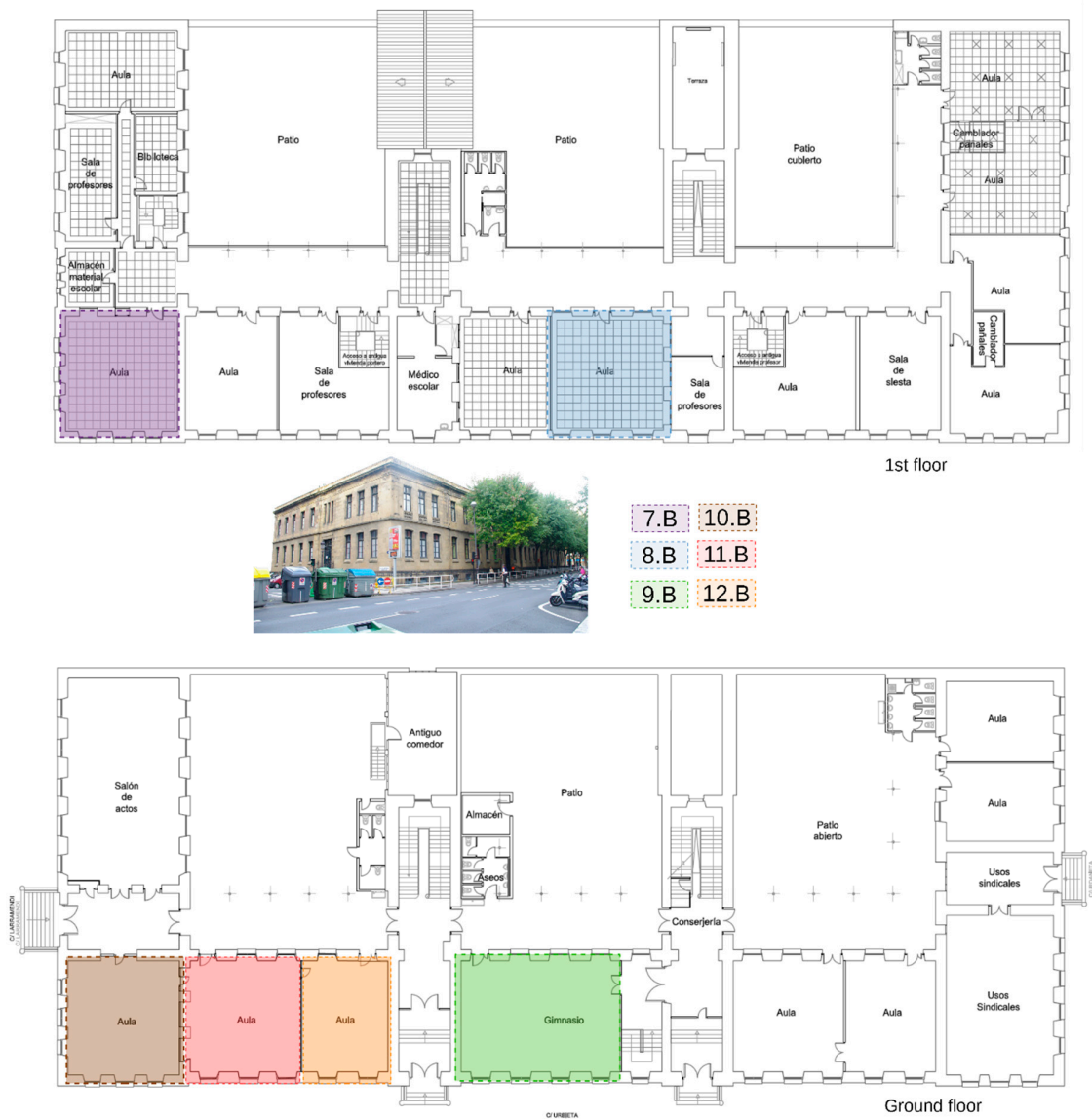
Figure A2. Floor plans of the blower door tests performed in the Urbieta School case study.
