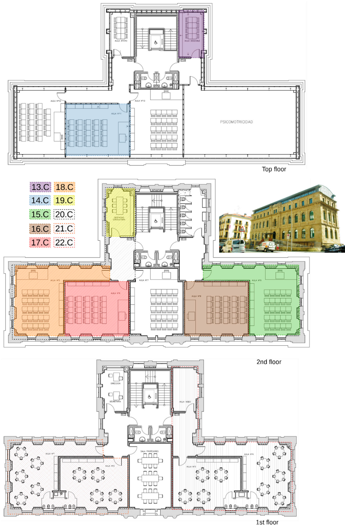
Figure A3. Floor plans of the blower door tests performed in the Aldamar School case study.
