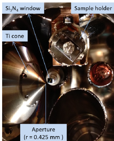
Figure 2.12. Picture of main chamber of APXPS system placed in beamline 9.3.2 at Advanced Light Source. The sample holder is a Thermionics STLC plate.
