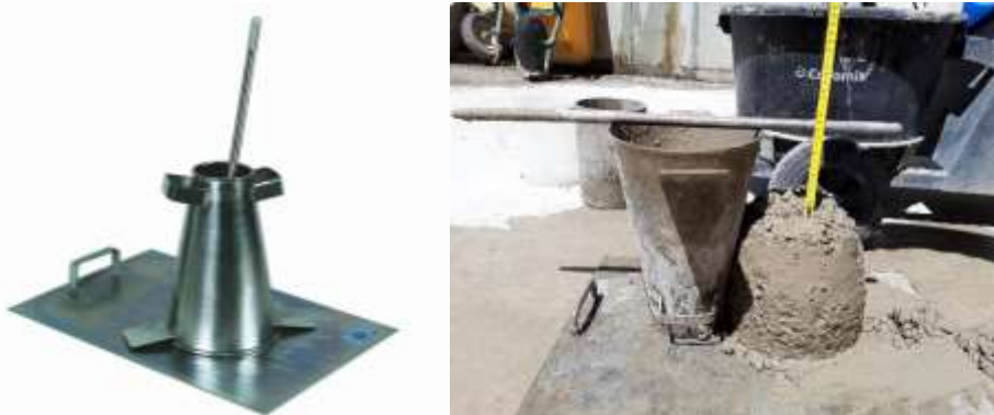
Fig. 5.6. Slump test with Abrams cone.
