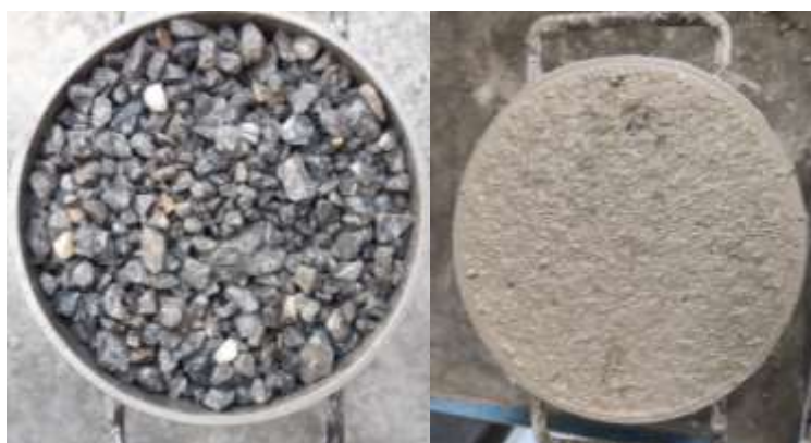
Fig. 4.29. Left: Appearance of the wet mix of NL (11/22) and NL (4/11); Right: Appearance of the wet mix of NL (11/22), NL (4/11) and NL (0/4).
