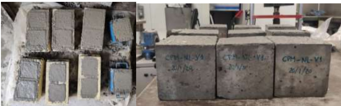
Fig. 5.8. Casting of concrete specimens.
