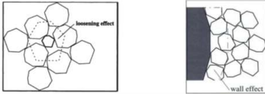
Fig. 4.10. Left: The loosening effect (coarse particles are dominant); Right: The wall effect (fine particles are dominant) (de Larrard 1999).
