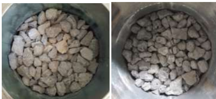
Fig. 4.13. Left: NL (11/22) fraction following D-C33 compaction within the cylindrical mould; Right: EAF (11/12) fraction following D-C33 compaction within the cylindrical mould.
