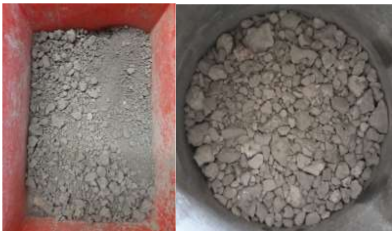
Fig. 4.31. Left: Mixture (0.4EC:0.60EM):0.4EF; Right: Appearance of the aggregate mixture following the D-C33 compaction process.
