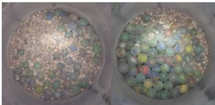
Fig. 4.25. The mixture of glass balls and fine rounded aggregate following compaction (0.5 by volume of each material). Left: D-C26 compaction process and Right: D-C33 compaction process.
