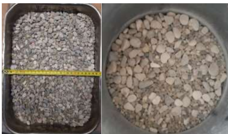
Fig. 4.23. Left: Mixing of the fine and coarse fractions (0.5 by volume) of rounded aggregates; Right: Aggregate mixture following the D-C26 compaction process.
