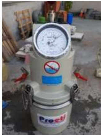
Fig. 5.7. Air entrainment meter, 8 l capacity.
