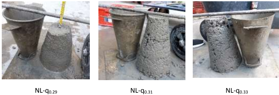
Fig. 5.20. Slump of the NL aggregate concrete mixes.
