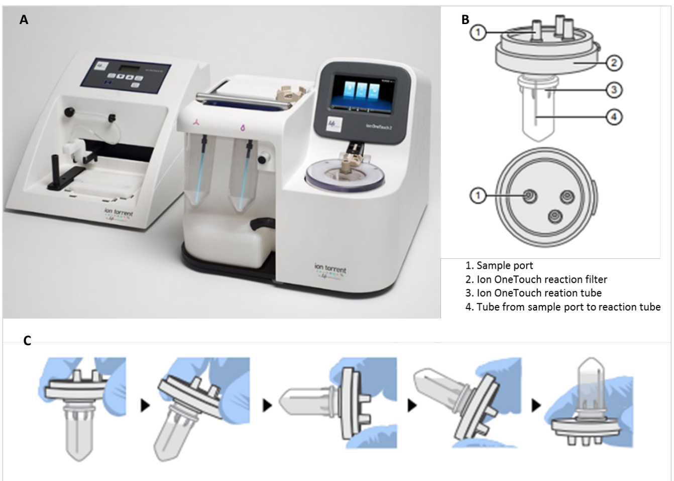
Figure 12. A, Image of the Ion OneTouch 2 system including the Ion OneTouch 2 instrument (right) and the Ion OneTouch ES instrument (left). B, Schematic representation of the Ion OneTouch reaction filter and C, its correct rotation with the amplification solution. Modified from Ion PGM™ Hi-Q™ OT2 Kit user guide.
