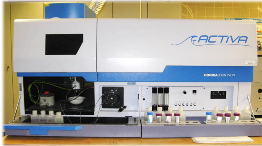
Figure A.22. Horiba Jobin Yvon Activa atomic emission spectrophotometer with inductively-coupled plasma (ICP-AES) from the SGiker (UPV/EHU).
