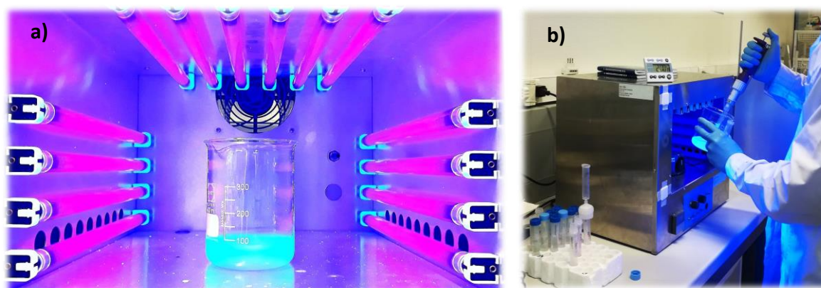
Figure A.18. LuzChem LZC-4V photoreactor (a) Inside and (b) outside during a photoreduction experiment with UVA light.
