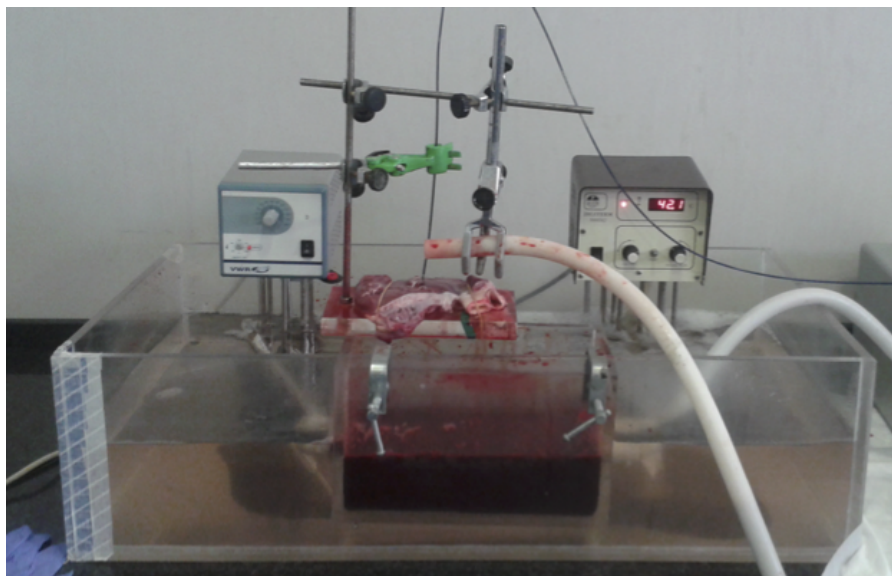
Figure 4.6: The experimental setup that we aim to reproduce with our model: the tissue and the electrode are submerged in a blood bath where blood flows thanks to a pump.
