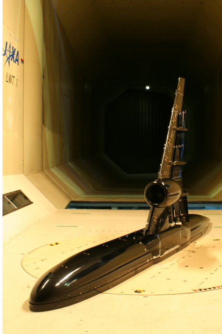
Figure 3.1: A model of the JSM aeroplane in a wind tunnel.
