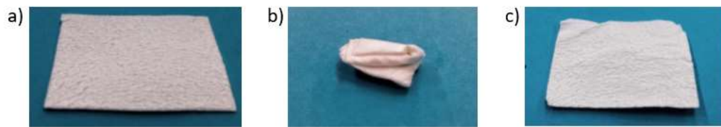
Figure 1.11 – Photographs of initial shape (a), fixed shape after folding the mat three times in half at 60 °C (b) and recovery shape after heating again to 60 °C (c). Reproduced with permission [109]. Copyright 2017, Elsevier.
