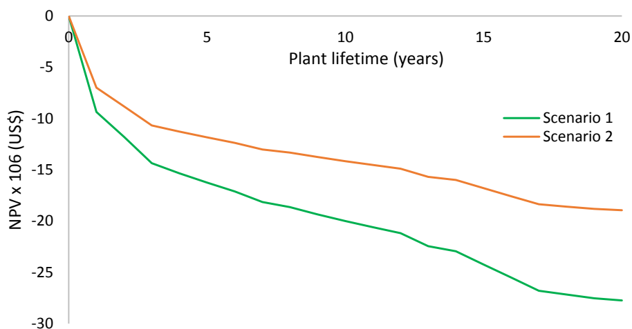
Fig. 2: Net Present Value of the P(3HB) production process over the project lifetime for both scenarios.
