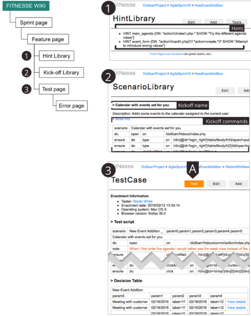
Figure 4.4: Wiki structure and distinct scaffolding pages for the Calendar application: Hint page (1), Kickoff page (2), and Test page (3). Test pages are enacted through the “ Test ” button (A).
