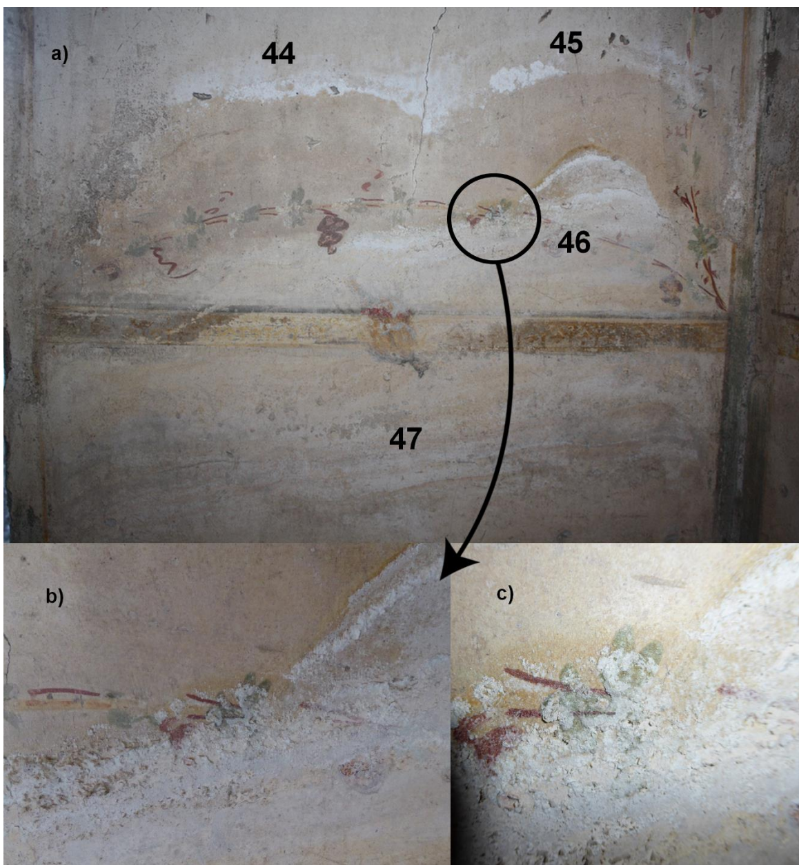
Fig. S18. A) Points GC_Q:44-47, analyzed by LIBS, HH-EDXRF and Raman spectroscopy at the eastern wall of Room Q of the House of the Golden Cupids. B) and C) Details of efflorescence GC_Q-46.
