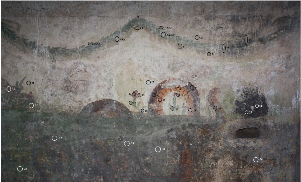
Fig. S3. Points (ARI_B:1-36) of the basement of the House of Ariadne analyzed by LIBS and HH-EDXRF.
