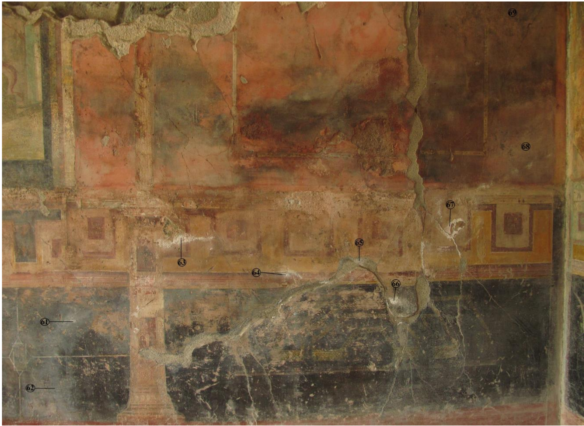
Fig. S6. Points (GC_G:61-69) of the northern wall of Room G of the House of the Golden Cupids analyzed by LIBS and Raman.
