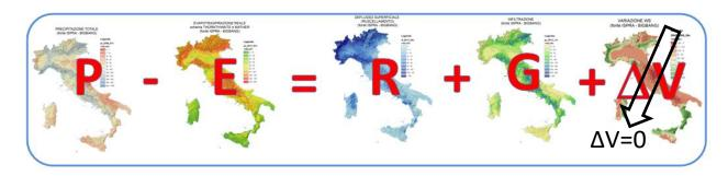
Figure 4. Equation of the hydrological balance
