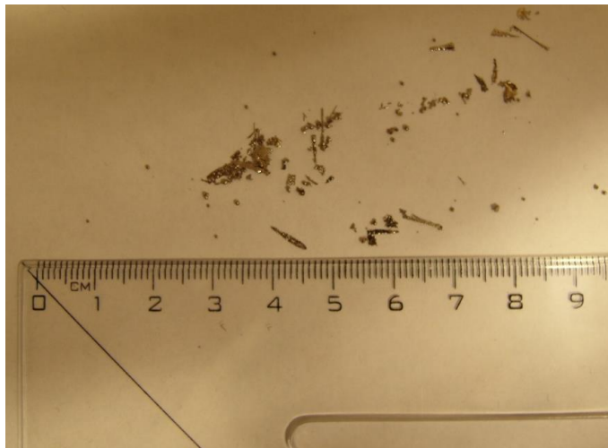
Fig. 41 Co 49 Ni 21 Ga 30 ribbon next to the ruler
