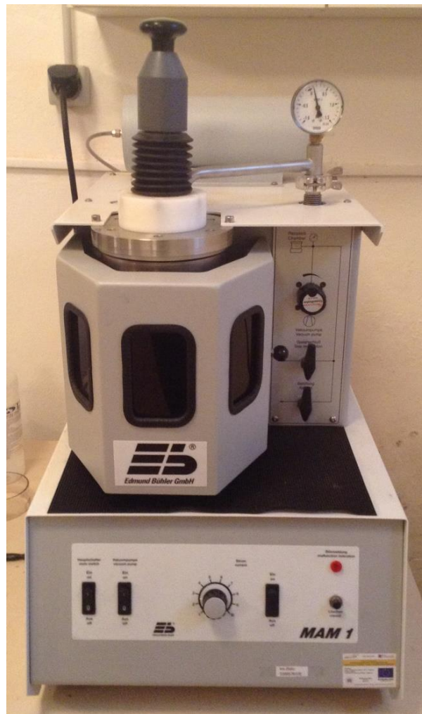
Fig. 29 Arc Melter MAM 1 with closed eye cover protection
