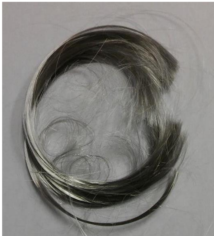
Fig. 61 Sample \text{Co}_{51}\text{Cr}_{17}\text{Ga}_{11}\text{Si}_{11} prepared by Taylor Ulitovsky method
