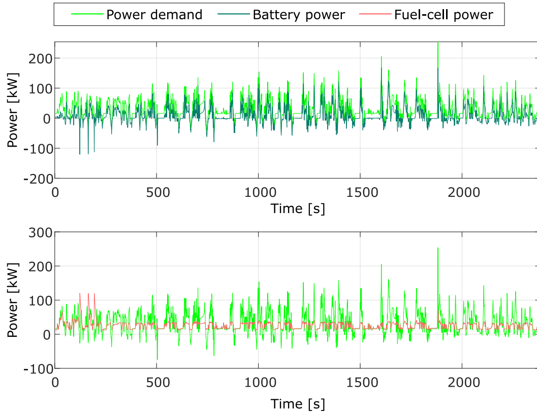
Figure 3.21: ANFIS based EMS power demand split between the BT (up) and the FC (down).
