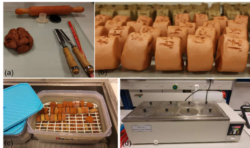
Figure 1. The manufacturing process of the test- and control-pieces before being fired. (a) the clay; (b) pieces before being fired; (c) test-pieces inside a seawater environment container; (d) the electric water bath containing the two environment containers.
