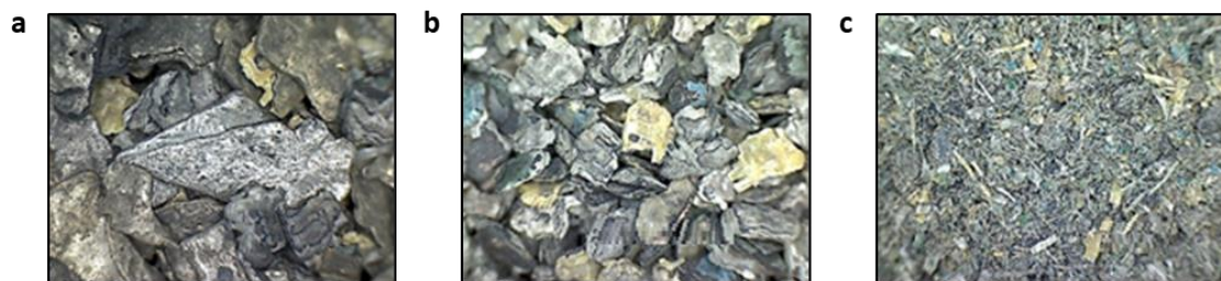
Figure 4.6. Pulverized PCB sample according to particle size: > 1.25 mm (a), 1.25-0.75 mm (b), and < 0.75 mm (c) (1:30 augmentation).
