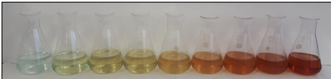
Figure 1.4. Color variation of the culture medium during the oxidation of \text{Fe}^{2+} into \text{Fe}^{3+} by means of A. ferrooxidans bacteria in 9K medium.
