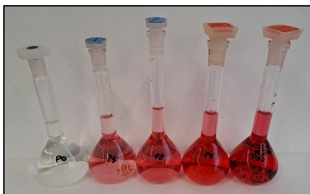
Figure 13. Iron standards for calibration curve.
