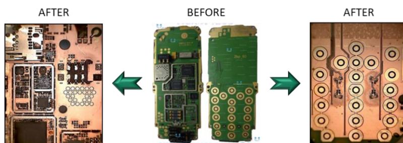
Figure 4.8. Mobile phone PCB before and after treatment with a 10 M NaOH solution.
