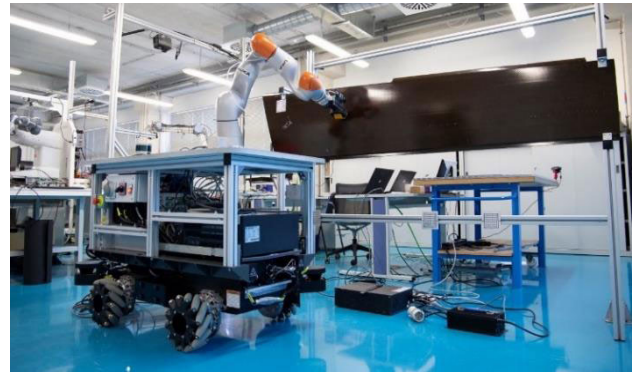
FIGURE 16. The robotic solution for advanced inspection of complex composite parts within the CRO-INSPECT project context.
