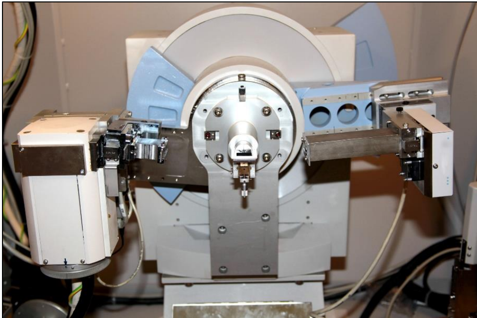
Figure 3.5. PANalytical Xpert PRO diffractometer for the X-Ray Diffraction of minerals
