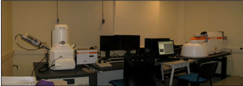
Figure 3.3. SEM-EDS instruments (left) coupled to an Invia Raman through the SCA interface (right)
