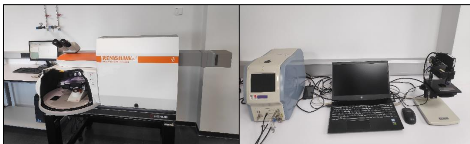
Figure 3.1. Raman instruments used in the development of this PhD thesis: Invia (left) and one of the InnoRam instruments (right)
