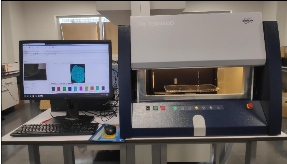
Figure 3.4. M4 Tornado for \mu -Energy Dispersive X-ray Fluorescence
