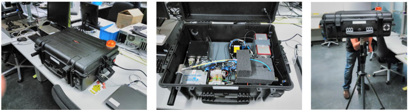
FIGURE 2. Packed prototype. (left) Acquisition case, (middle) Packed opto-mechanical system, (right) Tripod mounting.
