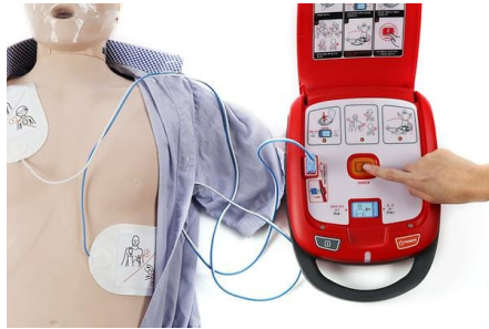
Figure 1.4. A commercial automated external defibrillator (AED) and the correct positioning of the defibrillation pads.
