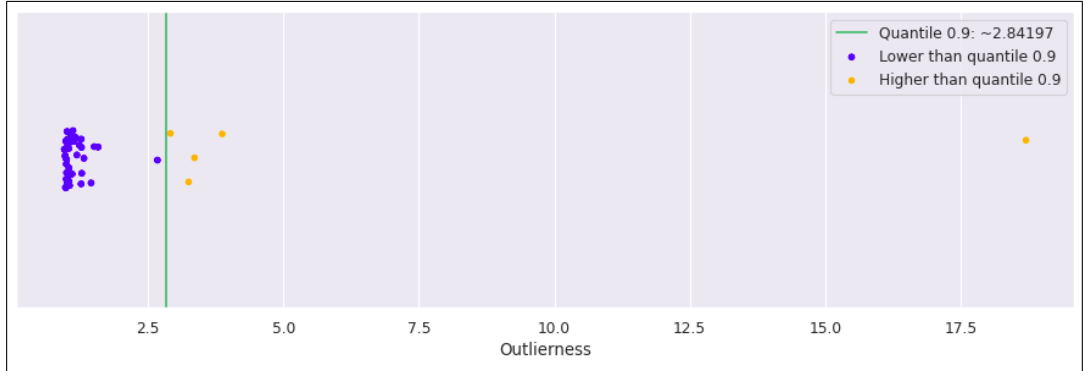
Figure 5.6: Example of outlierness analysis for sample filtering step in a certain fold of the 5-CV using LOF. The samples in yellow represent the cases whose outlierness is higher the one defined at quantile 0.9. It is clear how a large number of samples is gathered near 0 as expected, since the test subset is entirely made up of positive samples. However, there can be observed samples with higher outlierness that will eventually be labeled as outliers, and thus, removed from the train final subset.
