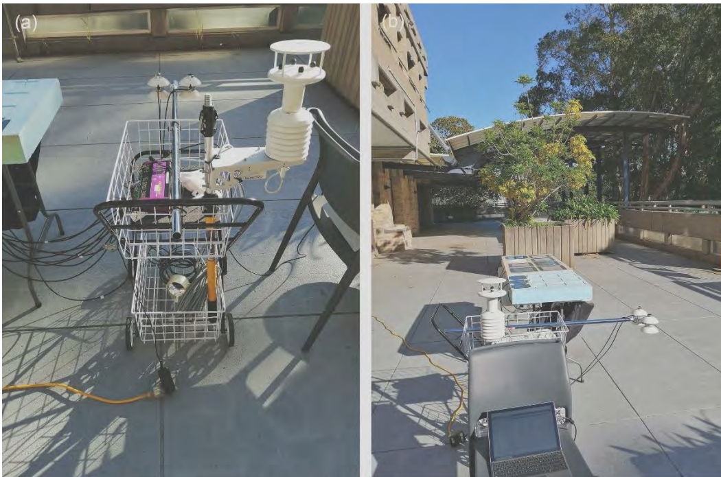
Figure 57: Photos of the experimental setup in the Square House at UNSW, Sydney, Australia. (a) Mobile meteorological weather station with radiometer (b) general photo of the samples contained in an XPS board and the weather station.
