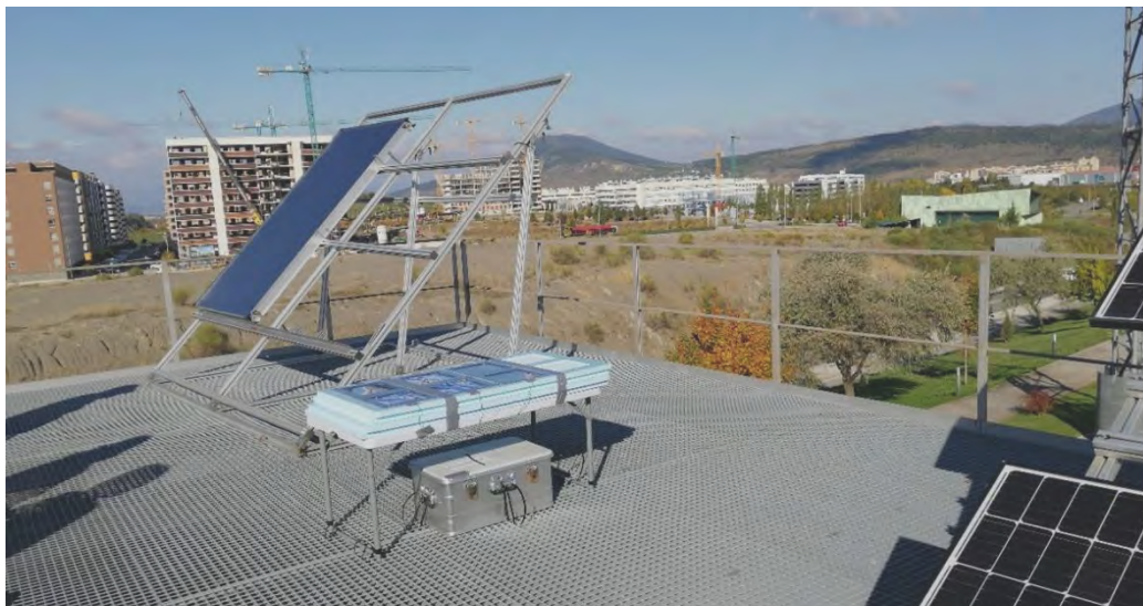
Figure 59: Photos of the experimental setup in CENER, Sarriguren, Spain. The samples are contained in an XPS board and monitored with thermocouples connected to dataloggers.
