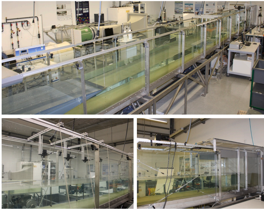
Fig. 1. Top: Overall view of the EWF of the Energy Engineering Department (UPV/EHU). Bottom: (left) Resistive-type wave probes and (right) piston-type wave generation system.
