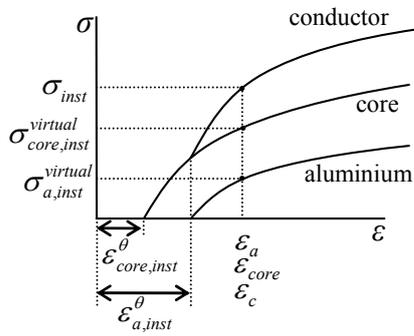
Fig. 8. Modified conductor stress-strain curve
