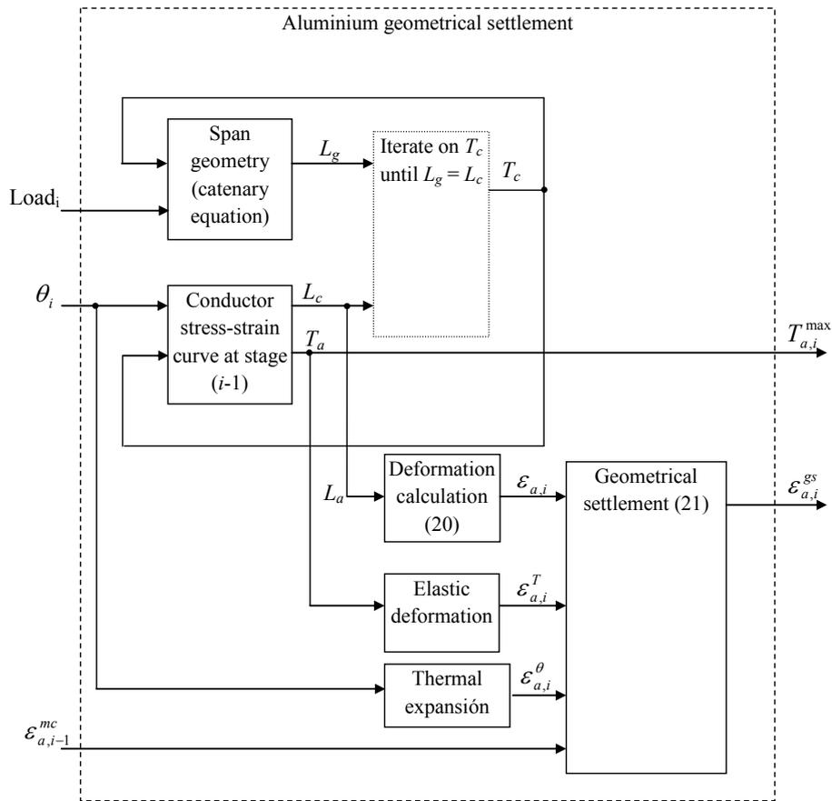
Fig. 10. Aluminium geometrical settlement calculation in the operation stage  $i$
