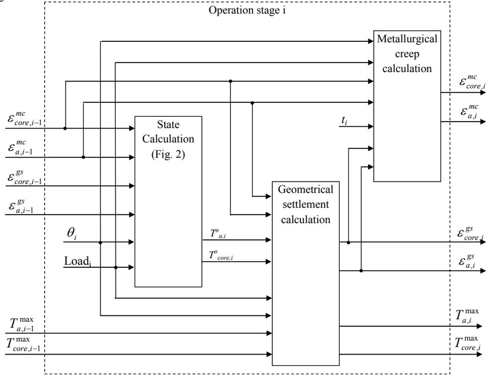
Fig. 9. Creep calculation in the operation stage  $i$
