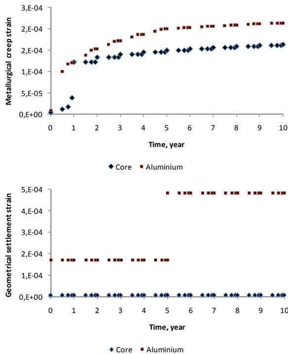
Fig. 12. Creep developed during the operation
