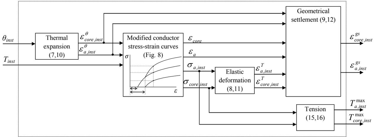
Fig. 7. Geometrical settlement creep developed in the core and the aluminium during the installation
