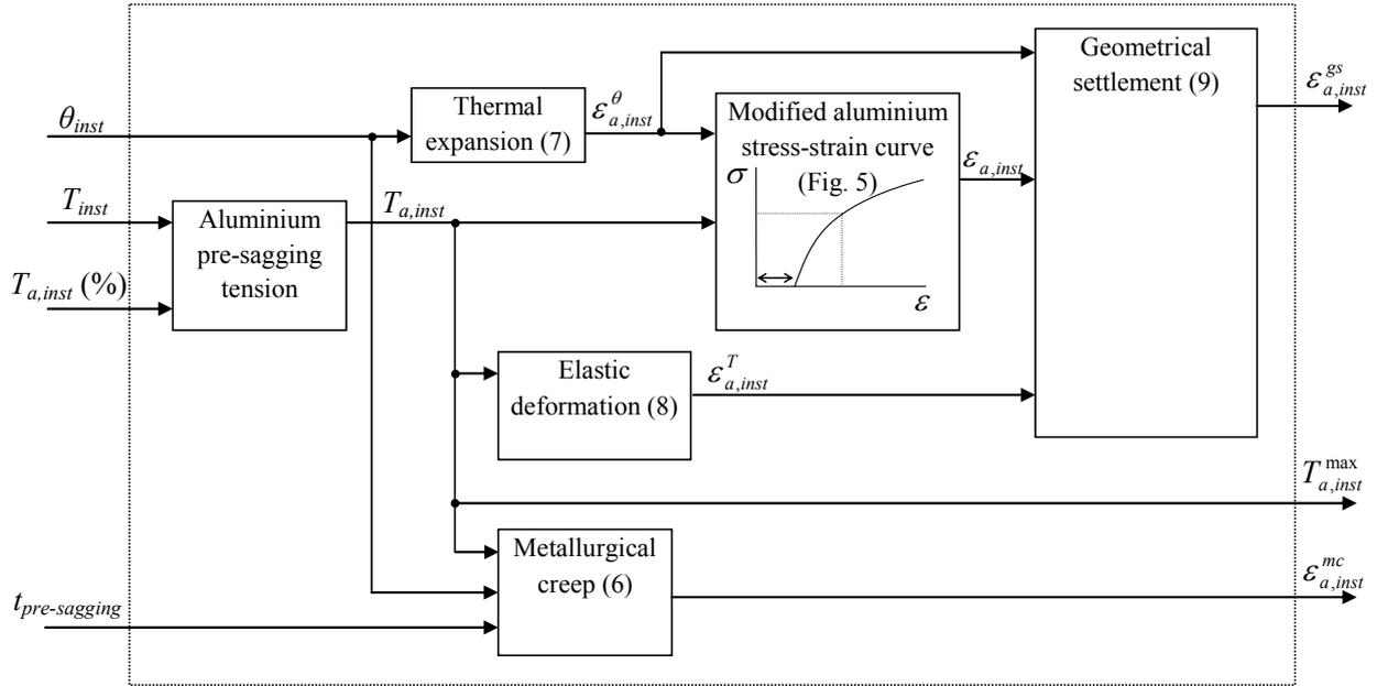
Fig. 3. Creep developed in the aluminium of a gap-type conductor during the installation
