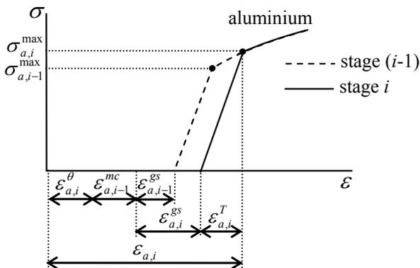
Fig. 11. Stress-strain curve of the aluminium at the end of the stages  $(i-1)$  and  $i$
