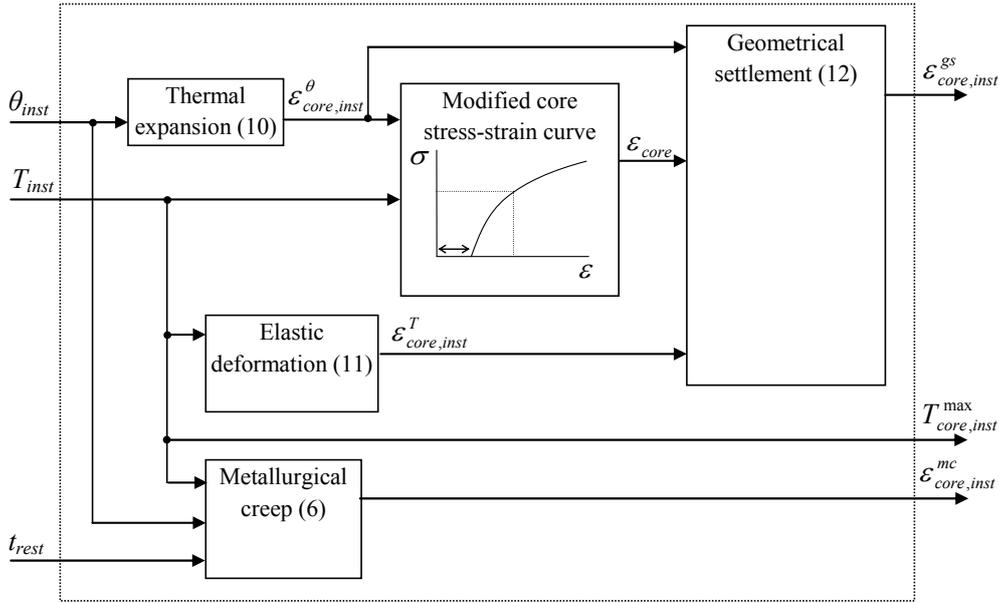
Fig. 6. Creep developed in the core of a gap-type conductor during the installation
