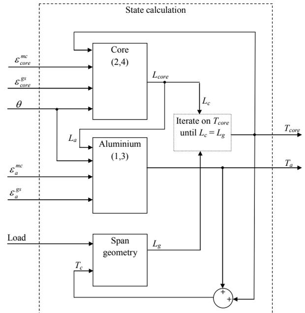
Fig. 2. State calculation algorithm
