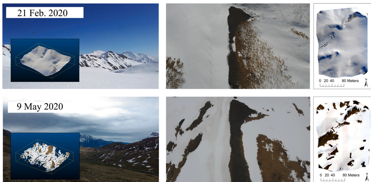
Fig. 6. Middle panel images: eBee Images of the same location corresponding to the first and second acquisition dates. Left side panel images: Point clouds generated with the images acquired with the Anafi UAV. These panels also depict two images of the study area acquired during the UAV flights, showing the sky conditions. Right panels show the orthophotos generated for each Anafi UAV flight.
