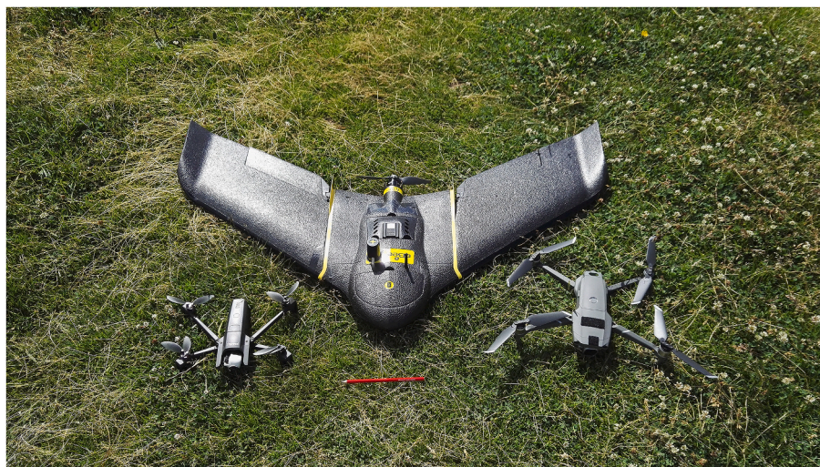
Fig. 3. Picture of the three UAV platforms tested in this work. Parrot Anafi on the left, Sensefly eBee Plus in the centre and DJI Mavic Pro 2 on the right.
