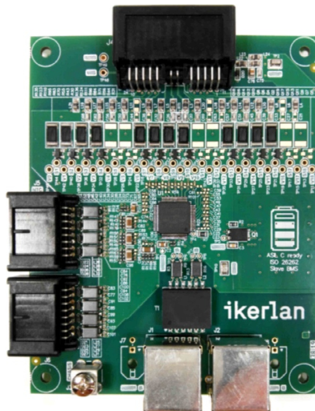
Figure 5. Developed enhanced battery management system slave prototype complying with functional safety ASIL C requirements.
