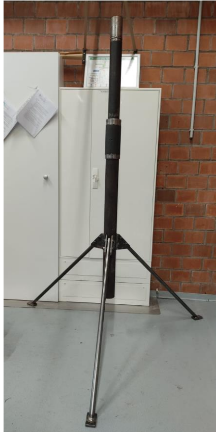
Figure 26 Manufactured tower of the wind turbine
