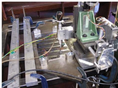
Fig. 1.7 Incremental drilling at strain gauge H4; plate bolted to mounting plate
