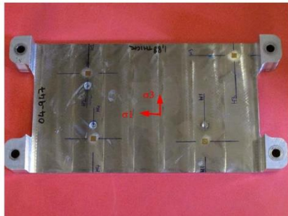
Fig. 1.3 Installation of strain gauges
