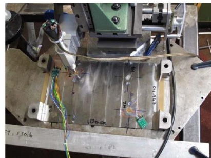
Fig. 1.8 Incremental drilling at strain gauge H1; plate cemented to mounting plate
