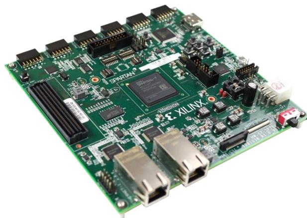
**Figura 37 Spartan-7 SP701 FPGA.**
