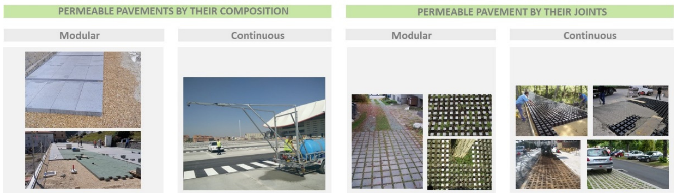
Figure A4. Types of green pavement (table and images by the authors, except images of continuous pavements [65,66]).
