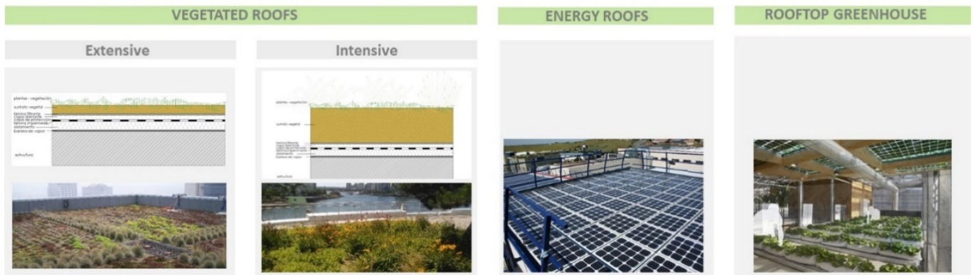
Figure A1. Types of green roofs (table and images by the authors).
