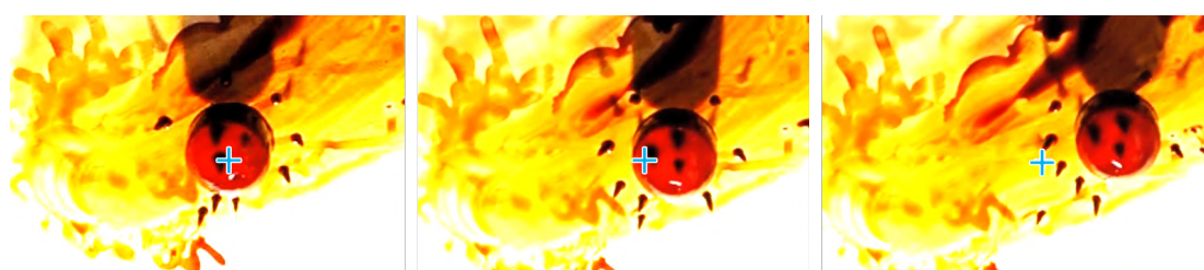
Figure 4.13: Manipulation of tSPRinged droplet on upside-down surface by translocation of the magnet. The cross sign shows the location of the droplet before manipulation.
